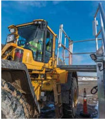
**The new loader steps make the job safer for operators. To view a video of the steps in action go to [www.transystemslc.com](http://www.transystemslc.com) or scan this code**
