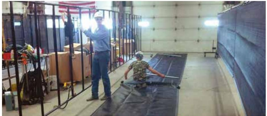
Above: Eric Boushey, EGF technician, stands ready to attach the new "monster mesh" while Gary Tvedt, a loader operator from Crookston, installs the cold roll into the mesh, which will enable him to clamp it onto the new gate.
