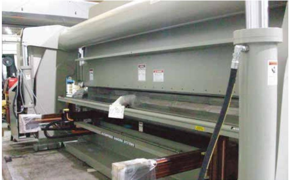
**The AccuPress 725020 allows the Manufacturing Project to bend nearly 90 percent of the parts needed to build trailers.**
